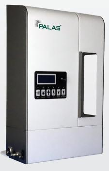
The **RBG** system fulfills these requirements for mass flows between 0.04 up to 800 g/h.
