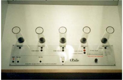
Three sniffing ports are used for the olfactory perception thresholds analysis. The odorous gas is brought to one of them while the two remaining ports are fed pure air. A random rotation of the odorous gas feed is assured by an algorithm. Using this method, jury members are subjected to a blind test.
