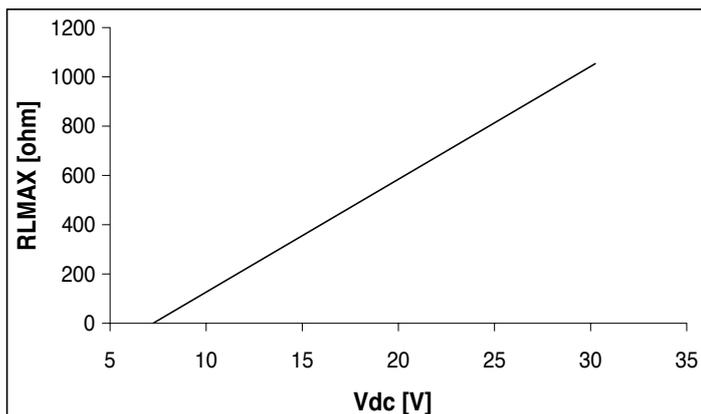
Fig. 3 Load with relation to the feeding voltage.
