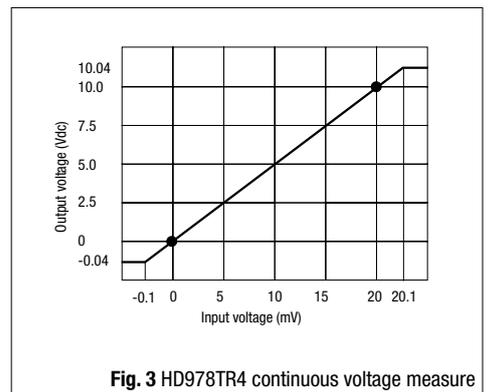
**Fig. 3 HD978TR4 continuous voltage measure**
