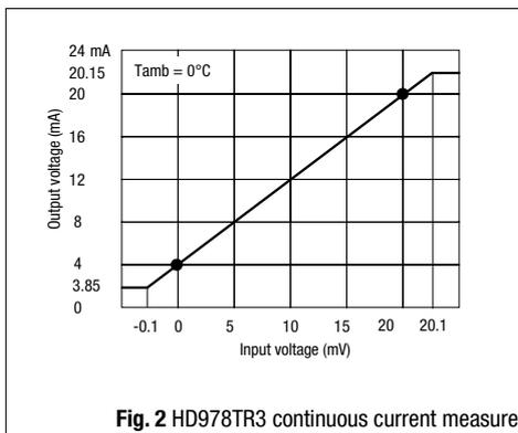
**Fig. 2 HD978TR3 continuous current measure**
