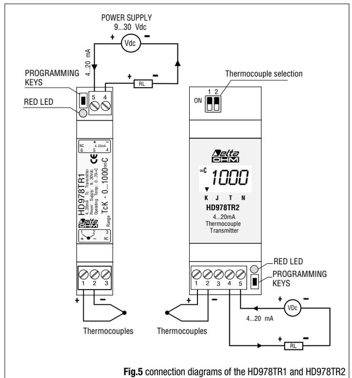
Fig.5 connection diagrams of the HD978TR1 and HD978TR2
