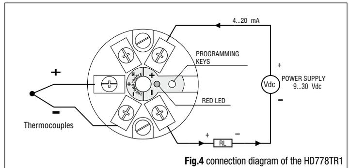
Fig.4 connection diagram of the HD778TR1
