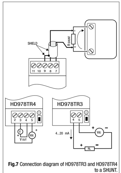
**Fig. 7** Connection diagram of HD978TR3 and HD978TR4 to a SHUNT.
