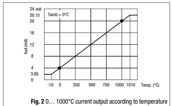
Fig. 2 0... 1000°C current output according to temperature
