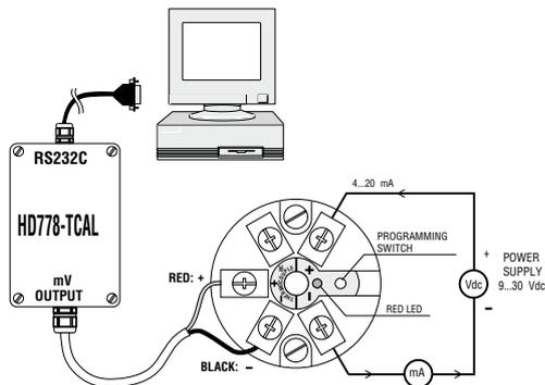
In place of the thermocouple calibrator, you can use the Delta Ohm **HD778-TCAL**: this instrument has to be connected to a serial port of the PC and, by means of a proper software, automates all the steps described below for programming the operating range.
