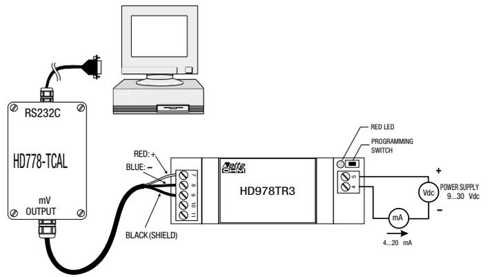
**current) or the HD978TR4 and HD978TR6 (0...10Vdc or 10...0Vdc voltage) by following the instructions on the screen.**
