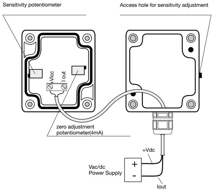
Figure 5. Connection diagram for HD2021T... with voltage output
