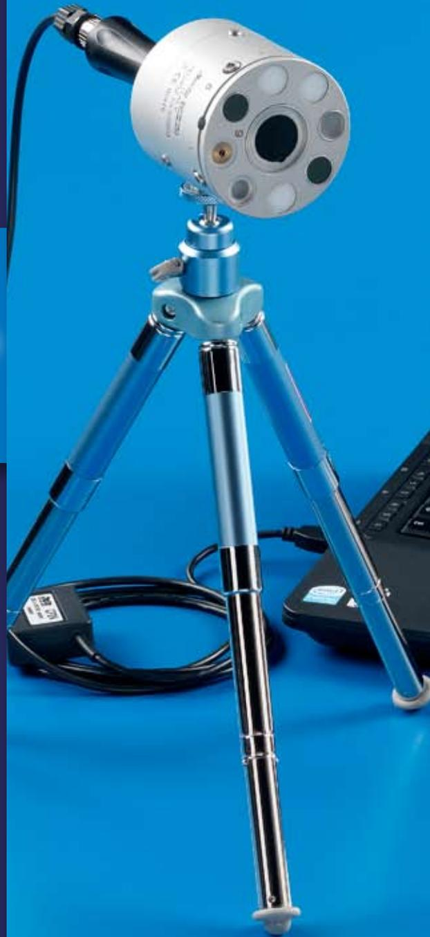
HD2402 is a portable photo-radiometer data logger for the measurement of non-coherent optical radiation in accordance with European Directive 2006/25/EC and the Legislative Decree No 81, April 9, 2008.
