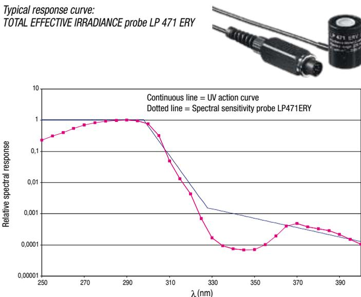
The probe LP 471 ERY measures the total effective irradiance (W<sub>eff</sub>/m<sup>2</sup>) according to the UV action curve (CEI EN 60335-2-27). A particular type of photodiode and a combination of special filters bring the spectral response closer to the UV action curve.
