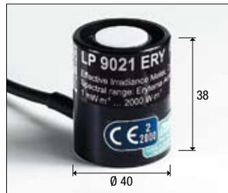
**LP 9021 ERY:** Radiometric probe for **TOTAL EFFECTIVE IRRADIANCE** ( $W_{\text{eff}}/m^2$ ) according to the UV action curve (CEI EN 60335-2-27) complete with SICRAM module. Spectral range: 250 nm...400 nm, quartz diffuser for cosine correction. Measurement range:  $0.1 \cdot 10^{-3} W_{\text{eff}}/m^2 \dots 2000 W_{\text{eff}}/m^2$ .
