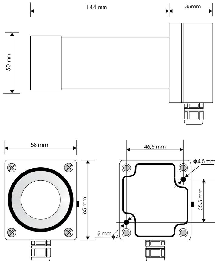
Figure 1. HD2021T6 probe dimensions
