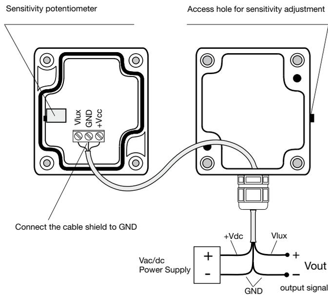
Figure 4. Connection diagram for HD2021T... with current output
