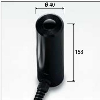
**LP 9021 LUM6:** Probe for measuring **LUMINANCE**, measuring range from 1 to 1999 x 10<sup>3</sup> candles/ m<sup>2</sup>. Measuring angle 2°. CIE filter for correction of the response according to the human eye, CIE n°69-UNI11142
