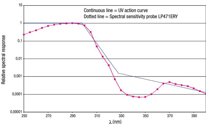
The probe LP 471 ERY measures the total effective irradiance (W<sub>eff</sub>/m<sup>2</sup>) according to the UV action curve (CEI EN 60335-2-27). A particular type of photodiode and a combination of special filters bring the spectral response closer to the UV action curve.
