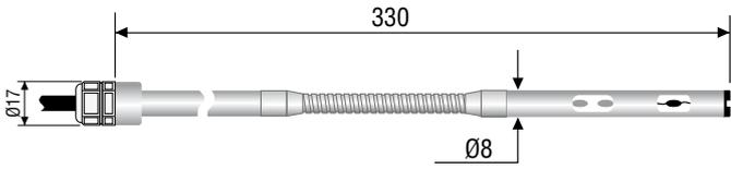
AP403S4 Omnidirectional probe for HD4...3TS4
