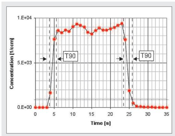
Measured concentrations for a stepwise concentration change at 0.6 lpm. The rise time of the CPCs in terms of T10-90 is below 3 s.
