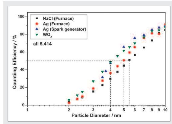
Efficiency of the CPC 5.414, measured with four different particle materials. A Faraday Cup Electrometer was used as reference (Rennecke 2010).
