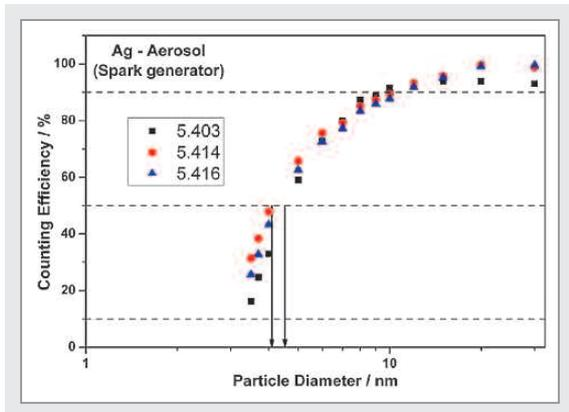
Counting efficiency as a function of particle size, measured with silver particles, for the CPCs 5.414 and 5.416. Both models feature the same new detection head. The efficiency of the mobile CPC 5.403 is shown for comparison. Data from Rennecke 2010.
