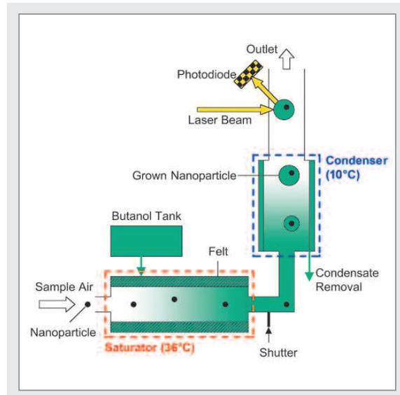
Schematic of a thermal diffusion – laminar flow CPC.
