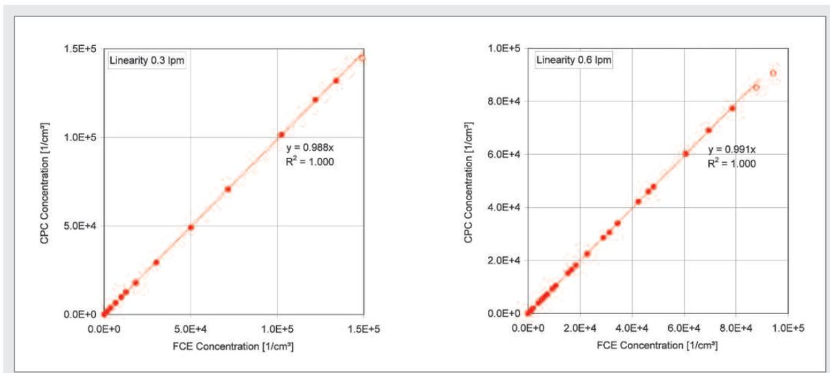
Linearity of the CPC in single count mode for a sample flow of 0.3 (left) and 0.6 lpm (right). Faraday Electrometer (FCE) concentrations serve as a primary standard.
