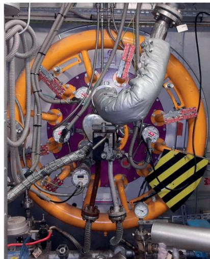
Pillard flame scanners fitted on industrial burners.
