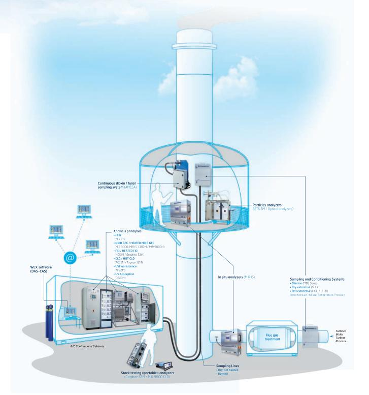
Vith many years of industrial experience, our turnkey systems are designed and engineered to provide a compl pproach from extraction of the sample, analysis, system build through the data acquisition and reporting. Each turnkey sy Illy configured to meet the ever-changing technical or regulatory needs of our industry or your company's ch
