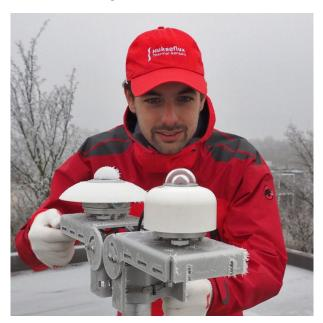
**Figure 3** frost and dew deposition: clear difference between a non-heated pyranometer (back) and SR30 with  $RVH^{TM}$  technology (front)
