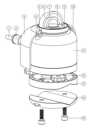
Figure 7 overview of SR30: (1) cable, (2) connector, (3) sun screen, (4) bubble level, (5) bubble level window, (6) outer dome, (7) inner dome, (8) thermal sensor with black coating, (9) internal ventilation vents, (10) quick release system of sun screen, (11) instrument body, (12) levelling feet, (13) optional spring-loaded levelling mount, (14) optional tube mount, (15) screws included with tube mount
