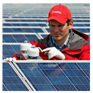
**Figure 6** SR30 secondary standard pyranometers with digital output for GHI (global horizontal irradiance) and POA (plane of array) measurement applications
