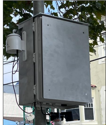
The microAeth® MA450 is a real-time 5-wavelength UV-VIS-IR Black Carbon monitor housed in an insulated outdoor enclosure with an 85 sampling location automatic filter tape advance system enabling 3-12 months of continuous measurements. The instrument includes the supports the DualSpot® loading compensation method which corrects for optical loading effects and provides additional information about aerosol optical properties.
